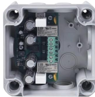
Loop isolator module, Part No. 583342
